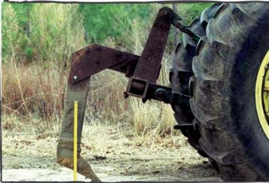
For compacted soils, a typical single shank subsoiler mounted on a tool bar should suffice for soil preparation.
